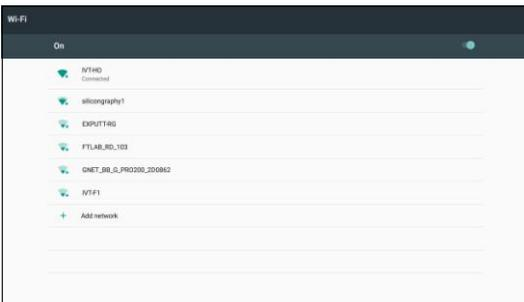
The Fig. on the left shows an image of the WIFI setup screen. Select the network you want to connect to and enter the password to complete network setup.
